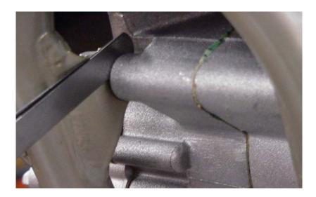
» In conjunction with carrying out the Engine Mounting Bracket Inspection, you also need to measure the width of the lower rear shock eye. It must not measure less than 23.80mm. If this measurement is less; you should replace both adaptor bushings (p.n. 46180007), which can also be ordered through the KTM Parts Distribution Center. » Submit a warranty claim for each motorcycle inspected using labor code T3900204970 for 20 minutes labor.
